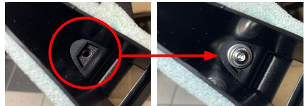
With the mount in place, turn everything upside down and take the supplied square nut and insert it into the small rectangular slot. Next, use the included hex wrench to fasten the screw and washer into the captured square nut, through the opening in the vent. Reinstall the vent nozzle with the new mount back into the dashboard to complete the installation.
