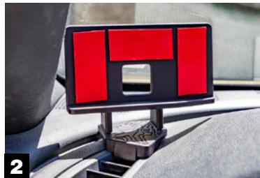
Remove the red film from the 3M heavy duty adhesive tape and attach the ScanGuage to the mount.
