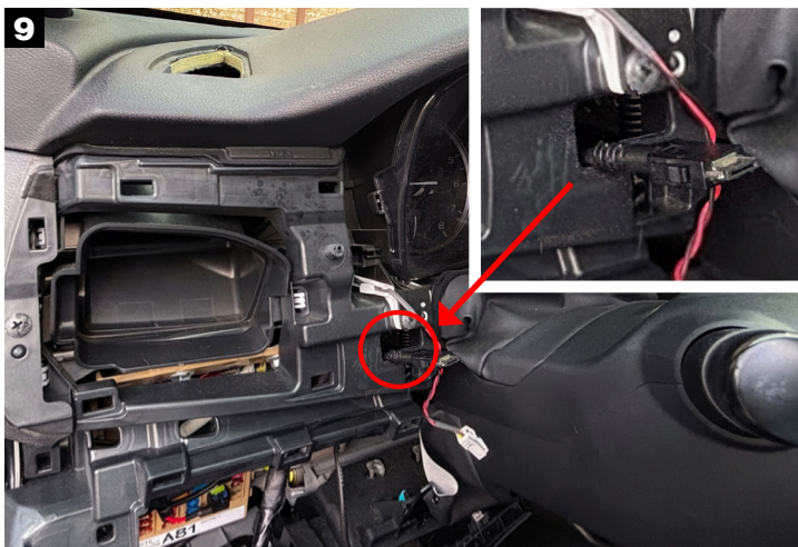
Run the Accessport data cable up through this opening.
