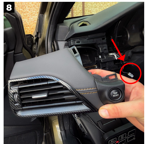
Unclip the left AC vent. It releases relatively easily. You will need to remove the connector from the Trip Reset switch.
