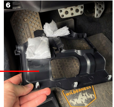
Unclip this panel from directly under the dashboard.
