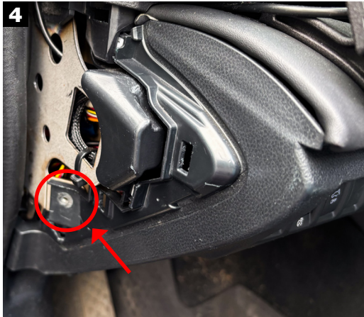
Once the panel is removed, use a phillips head screwdriver to remove the screw.
