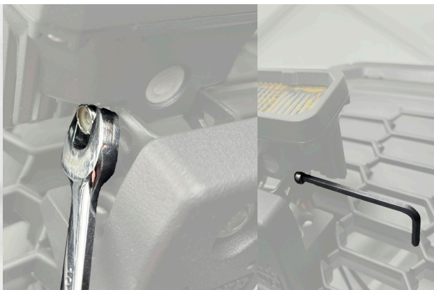
5 Using a 10mm wrench and the included 4mm hex wrench, install the SS2 fog light onto the kit's bracket
