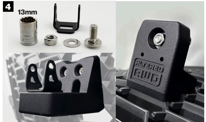
4 Using a 13mm socket and the hardware that comes with your SS2 fog lights (carriage bolt, washer, and nut) install the bracket on the front mount. Ensure the bracket is facing in the same direction as the image above.
