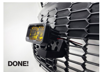
6 The wires for the fog light will run cleanly through the grille, past the new mount.
